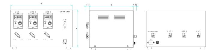
CUBE GM2 : W315×D298×H250(mm)%Not including protrusions.CUBE GM3 : W415×D298×H250(mm)%Not including protrusions.CUBE GM4 : W515×D298×H250(mm)%Not including protrusions.
